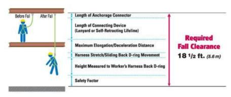
Allow the minimum calculated clearances necessary above the ground, equipment, or other obstruction at the end of the fall from the fall arrest point.
